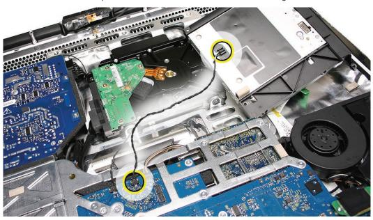
Replace the T6 screws on the optical flexible cable.
